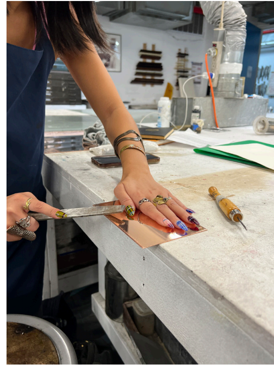
1. Vivian prepared the plate by using a flat file to bevel the edges, which prevents the plate from tearing the paper as it is pulled through the pressure of the printing press.
