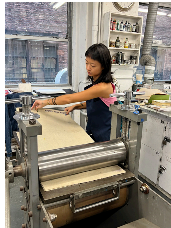
6. After the plate had been cleaned, inked, and excess ink wiped away, Vivian turned to the printing press to pull the print. The plate was positioned face up on the press bed, and slightly dampened paper was centered on the metal surface. The blanket was laid over the plate and paper to evenly distribute pressure as they were mechanically pulled through the rollers.
